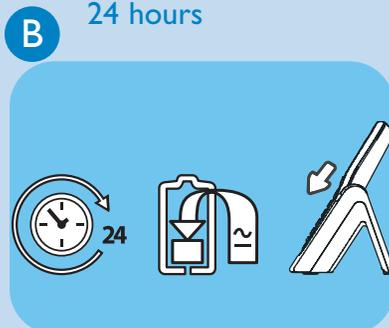
If the batteries are completely exhausted, the handset will not be able to power-on immediately. Handset may get warm during initial charge. This is normal.
