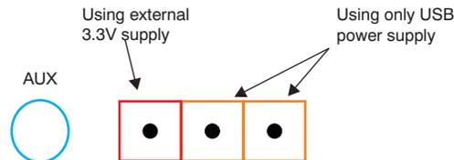
Figure 8. JP1 Setting for USB Programming Configuration
