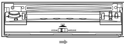
4. Push and slide the DCP upward to remove.
