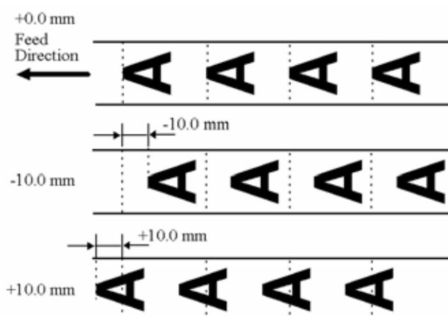
**NOTE:** The fine adjustment value equals to the sum of the fine adjustment values set by the PC command and this parameter.
