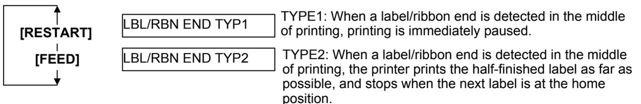
After selecting a Label End/Ribbon End type, press the **[PAUSE]** key.
