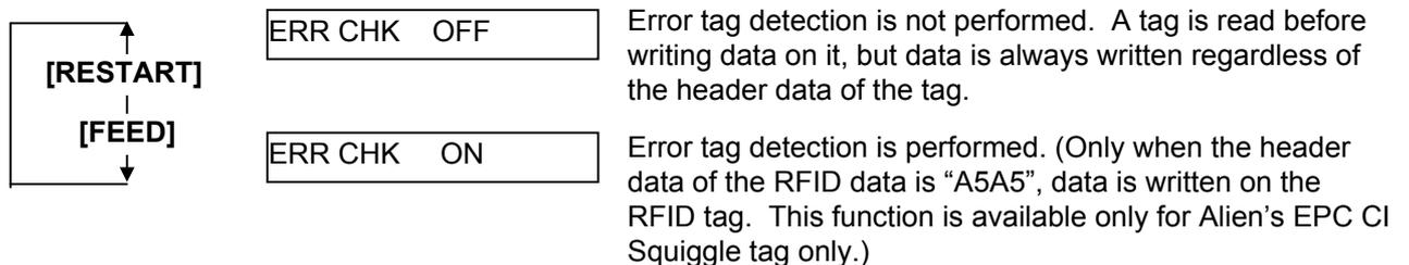
After selecting the RFID error tag detection function to be used, press the **[PAUSE]** key.
