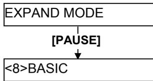
When the program for the Basic expansion mode has been downloaded, it will be executed by pressing the **[PAUSE]** key. The way of completion is different depending on the program.
