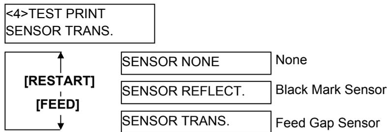
After selecting a sensor type, press the **[PAUSE]** key to go to Printing Mode Selection.
