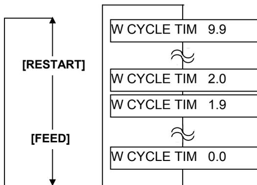
**[FEED]** key: Pressing the **[FEED]** key one time causes a  $-0.1$  change, up to 0.0.
