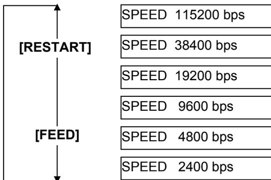
After selecting a baud rate, press the **[PAUSE]** key.
