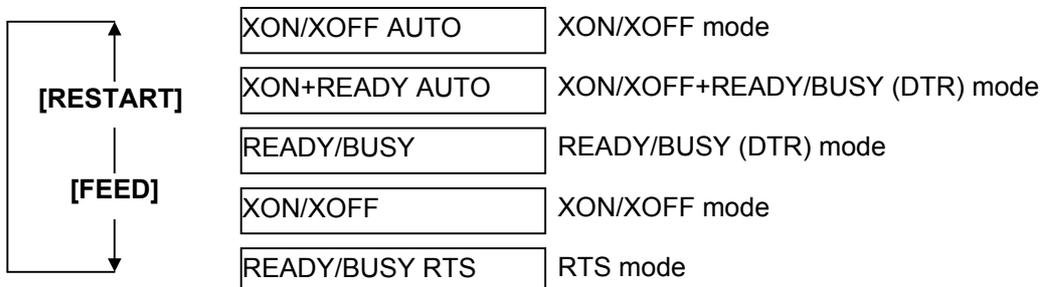
After selecting a flow control code, press the **[PAUSE]** key.
