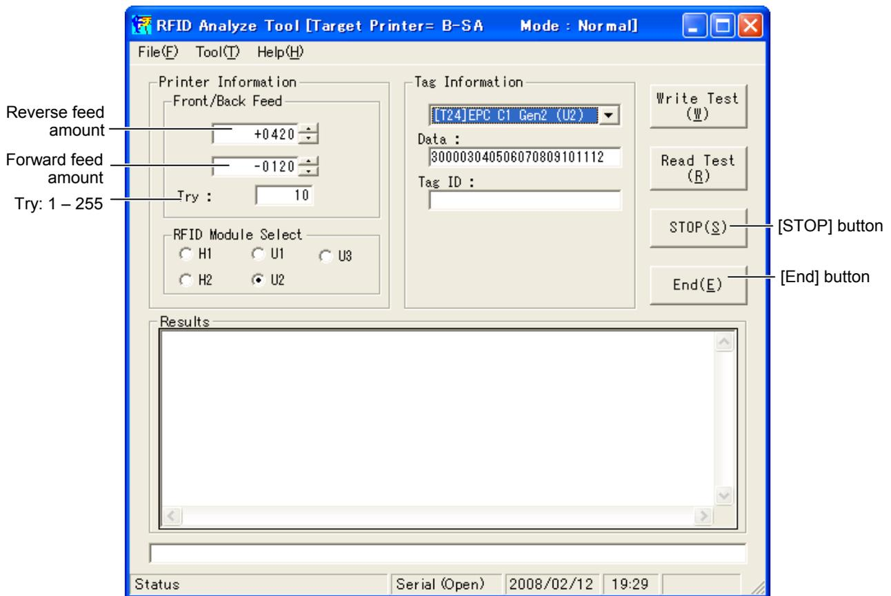
5. Perform a write test or read test.
