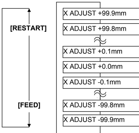
**[FEED]** key: Pressing the **[FEED]** key one time causes a  $-0.1$  mm change, up to  $-99.9$  mm.
