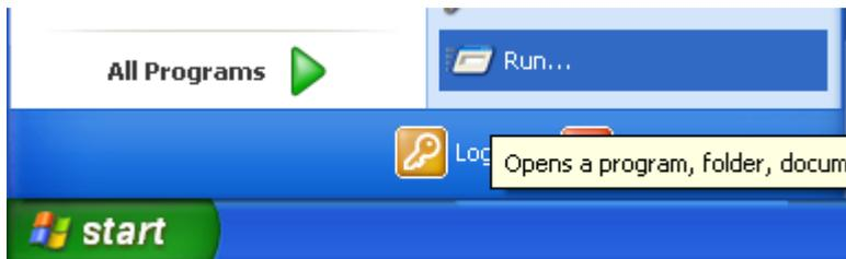
3. When the “Run” screen appears, enter “D:\Setup.exe” in the “Open” entry field, then click on the “OK” button. (When the CD-ROM drive is drive D.)
