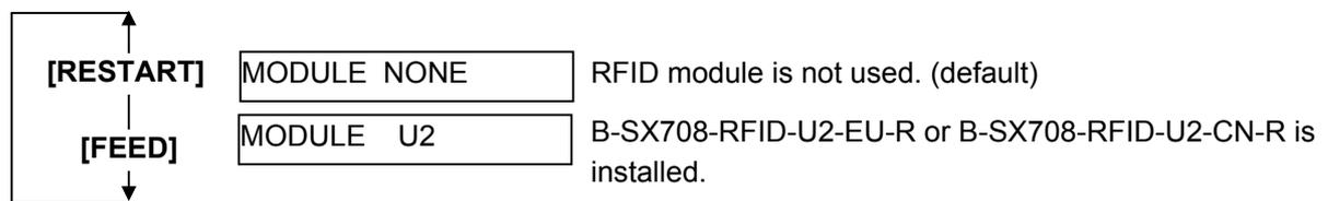
**NOTE:** This parameter setting is effective when turning OFF then ON the printer.
