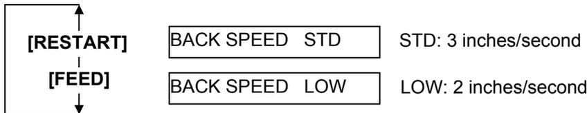
After selecting the Back Feed Speed, press the **[PAUSE]** key.
