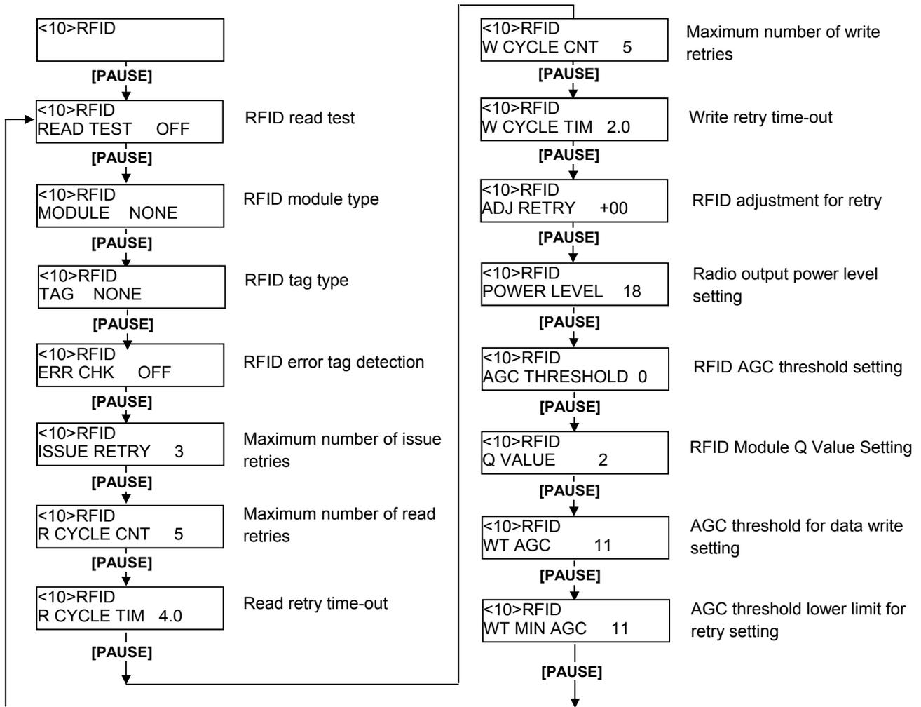
■ **How to Enter RFID Module Setting Mode**
