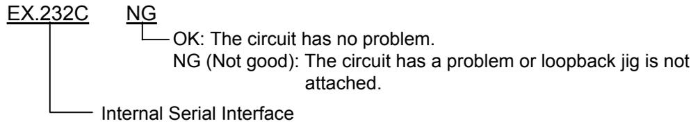
Connect the jig like below to the serial interface connector and perform a loop back check.
