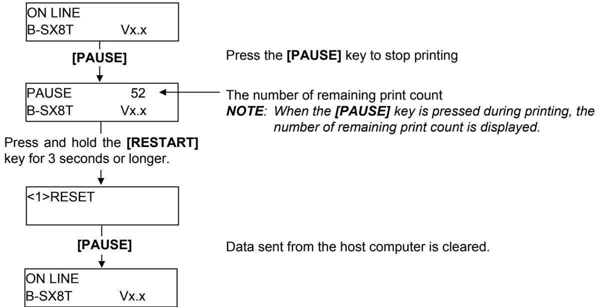
**NOTE:** Failure to press the **[RESTART]** key for 3 seconds or longer causes the printer to restart printing. However, when a communication error or command error occurs, the printer returns to an idle state.
