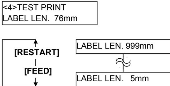
**[FEED]** key: Pressing the **[FEED]** key one time causes a –1 mm change, up to 5 mm.
