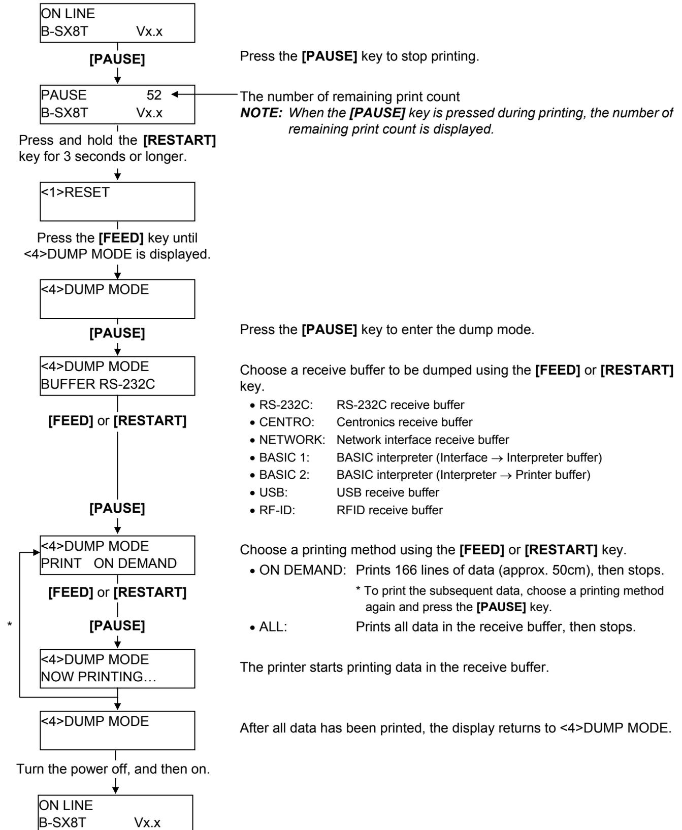
The data in the receive buffer is printed as follows:
