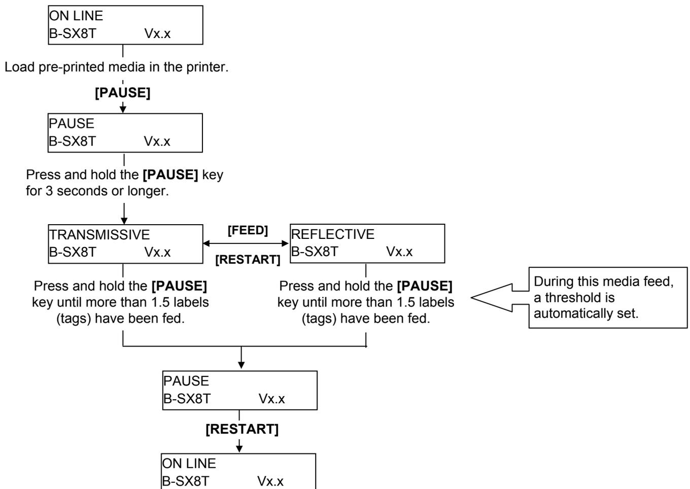
**NOTES:** 1. Failure to feed more than 1.5 labels may result in an incorrect threshold setting.
