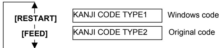
**NOTE:** Kanji code selection is not supported by the QM model as the Kanji ROMs are not installed.
