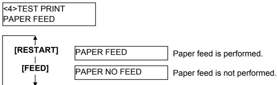
After selecting whether to perform a paper feed, press the **[PAUSE]** key. The display returns to the "<4>TEST PRINT".
