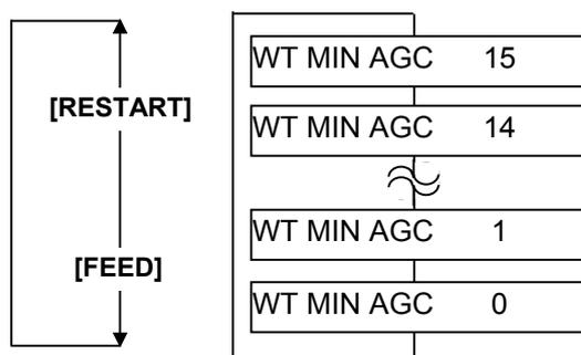
After selecting the adjustment value, press the **[PAUSE]** key. The display returns to "<10>RFID".
