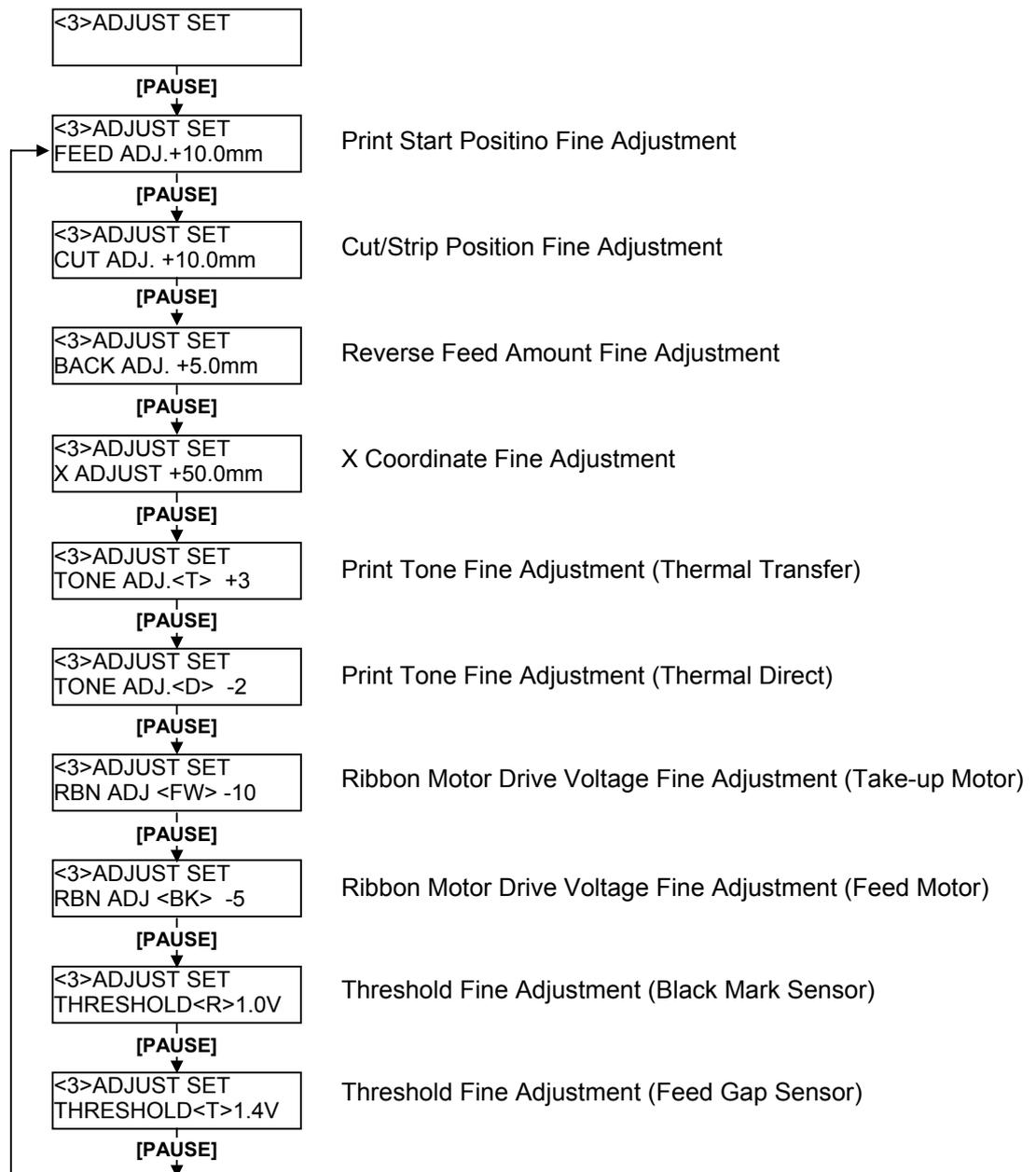
**■ How to Enter Printer Parameter Fine Adjustment Mode**
