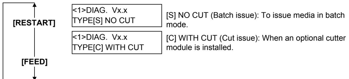
**NOTE:** When using the cutter module, be sure to select “[C] WITH CUT”. When the cutter module is not installed, be sure to select “[S] NO CUT”.
