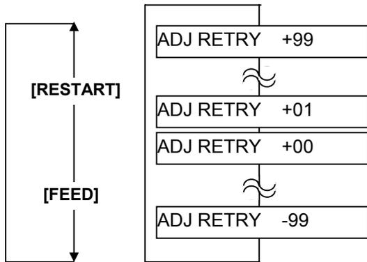
**[FEED]** key: Pressing the **[FEED]** key one time causes a -1mm change, up to -99mm.
