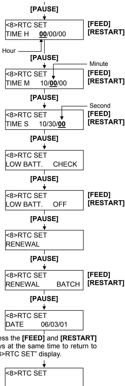
Press the **[FEED]** and **[RESTART]** keys at the same time to return to “<8>RTC SET” display.
