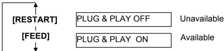
**NOTE:** If the printer and the PC are connected by USB, plug & play will be automatically enabled, regardless of the setting of this parameter.
