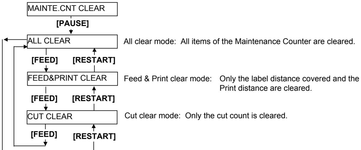
After choosing a mode, press the **[PAUSE]** key. A maintenance counter clear will be performed according to the chosen mode.
