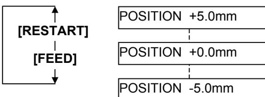
**[FEED]** key: Pressing the **[FEED]** key one time causes a  $-0.1$  mm change, up to  $-5.0$  mm.
