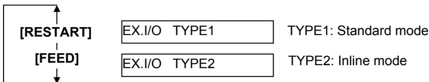
After selecting an Expansion I/O Interface type, press the **[PAUSE]** key.
