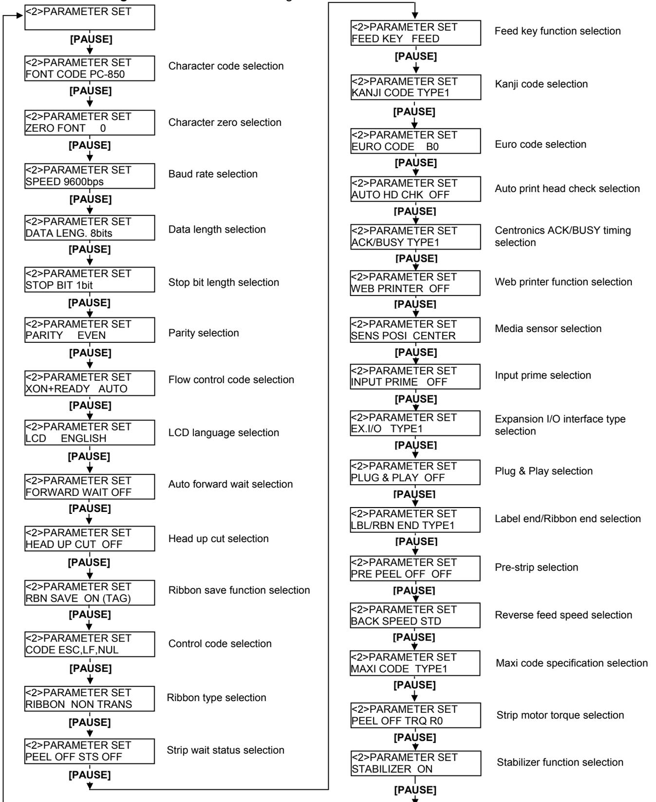
**NOTE:** Baud rate, Data length, Parity, and Transmission control code should be set to the same values as those of the host computer. Failure to do this causes improper operation.
