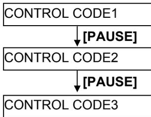
Press the **[PAUSE]** key after setting the control code for Control Code 3.
