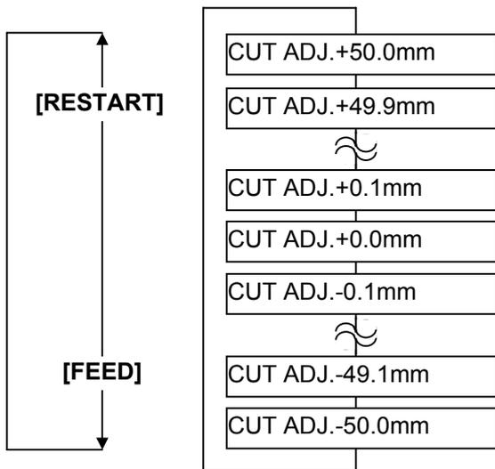
[FEED] key: Pressing the [FEED] key one time causes a -0.1 mm change, up to -50.0 mm.
