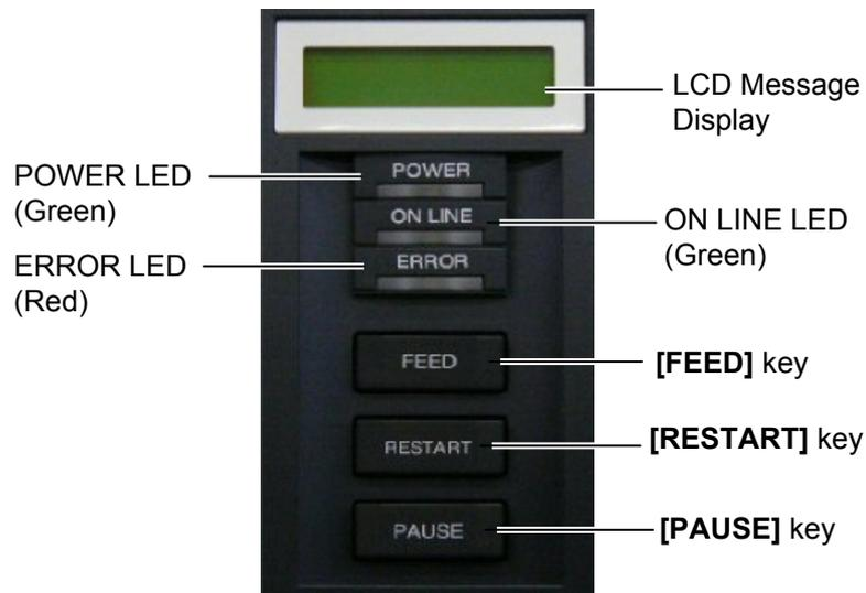
The LCD Message Display is a 16-character x 2-line display, which shows messages in alphanumeric characters and symbols to indicate the printer's status. .
