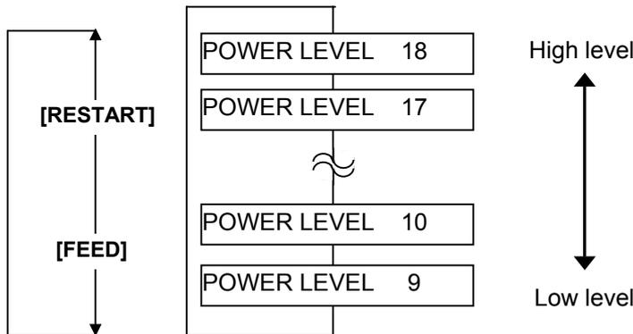
After selecting the adjustment value, press the **[PAUSE]** key. The display returns to "<10>RFID".
