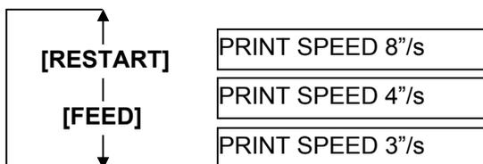
After selecting a print speed, press the **[PAUSE]** key to go to Sensor Type Selection.
