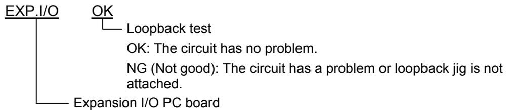
Connect the jig like below to the Expansion I/O PC board's connector and perform a loop back check.
