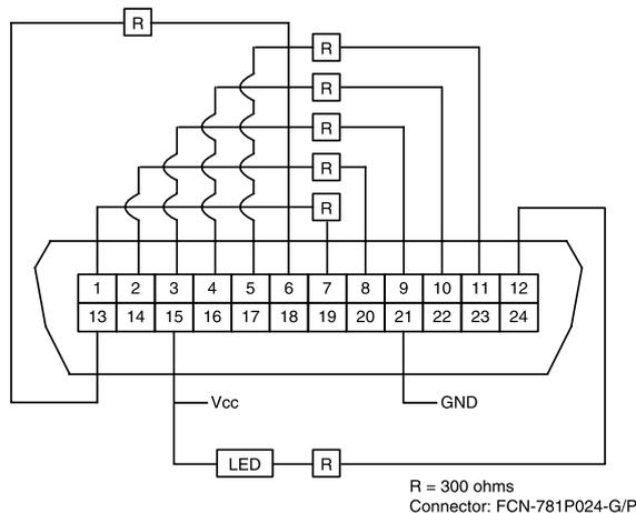
(11) Internal Serial Interface Check
