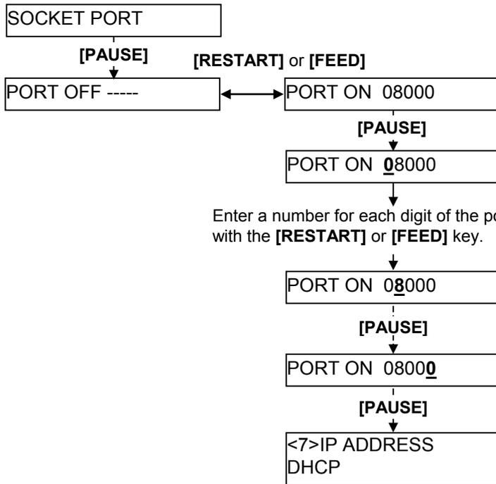
Enter the 5th digit of the port number with the [RESTART] or [FEED] key. Pressing the [PAUSE] key allows the 4th digit setting. Repeat this procedure until the 1st digit setting has been completed.
