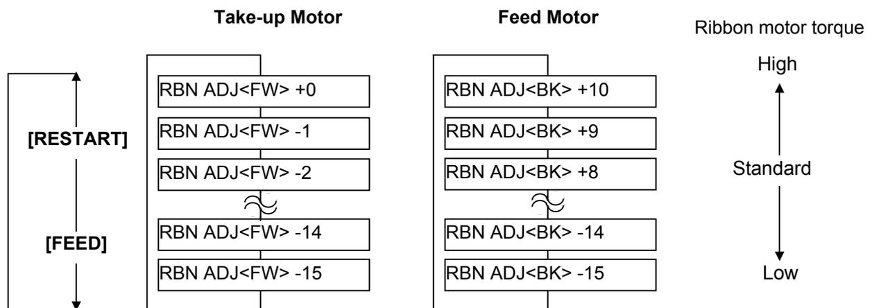
**[FEED]** key: Pressing the **[FEED]** key one time causes a -1 step change, up to -15 steps.
