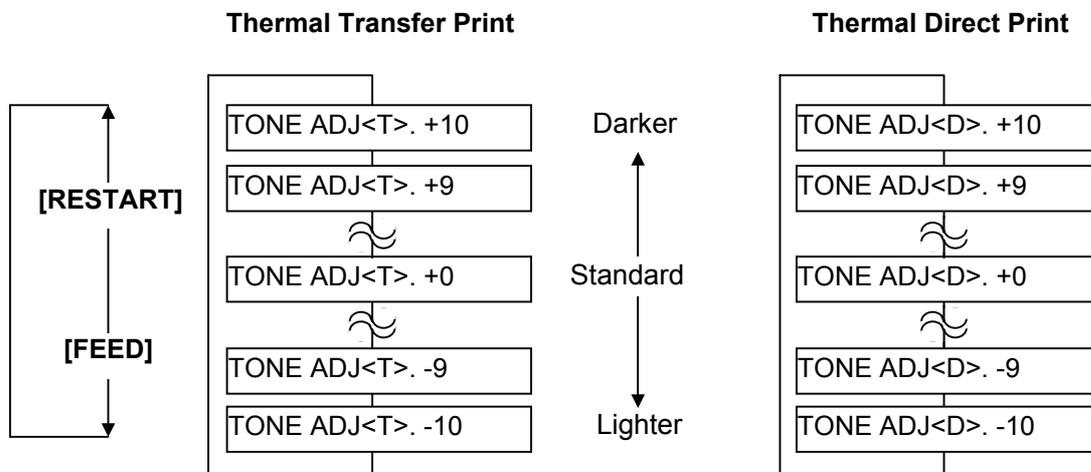
**[FEED]** key: Pressing the **[FEED]** key one time causes a -1 tone change, up to -10 tones.
