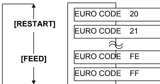
**NOTE:** Pressing the **[FEED]** or **[RESTART]** key causes 1 byte change in the Euro Code value.
