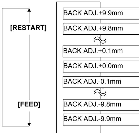
**[FEED]** key: Pressing the **[FEED]** key one time causes a -0.1 mm change, up to -9.9 mm.
