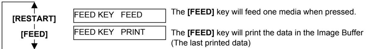
After selecting the FEED key function, press the **[PAUSE]** key.
