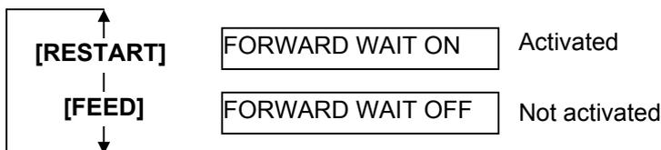
When ON is selected, pressing the **[PAUSE]** key will result that the LCD Message Display shows the stop position fine adjustment value setting screen.
