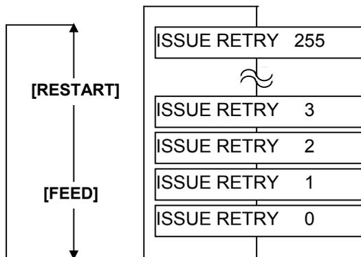
**[FEED]** key: Pressing the **[FEED]** key one time causes a –1 change, up to 0.
