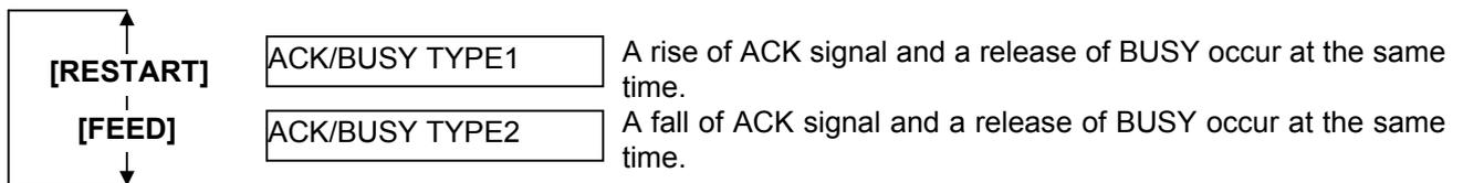
After selecting an ACK/BUSY timing, press the **[PAUSE]** key.
