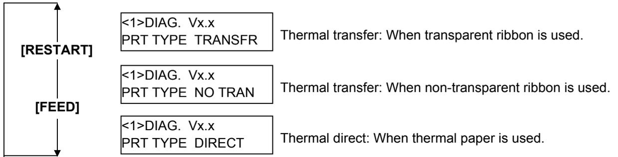
**NOTE:** When using the ribbon, be sure to select “Thermal Transfer”. When using the thermal media, be sure to select the “Thermal Direct”.
