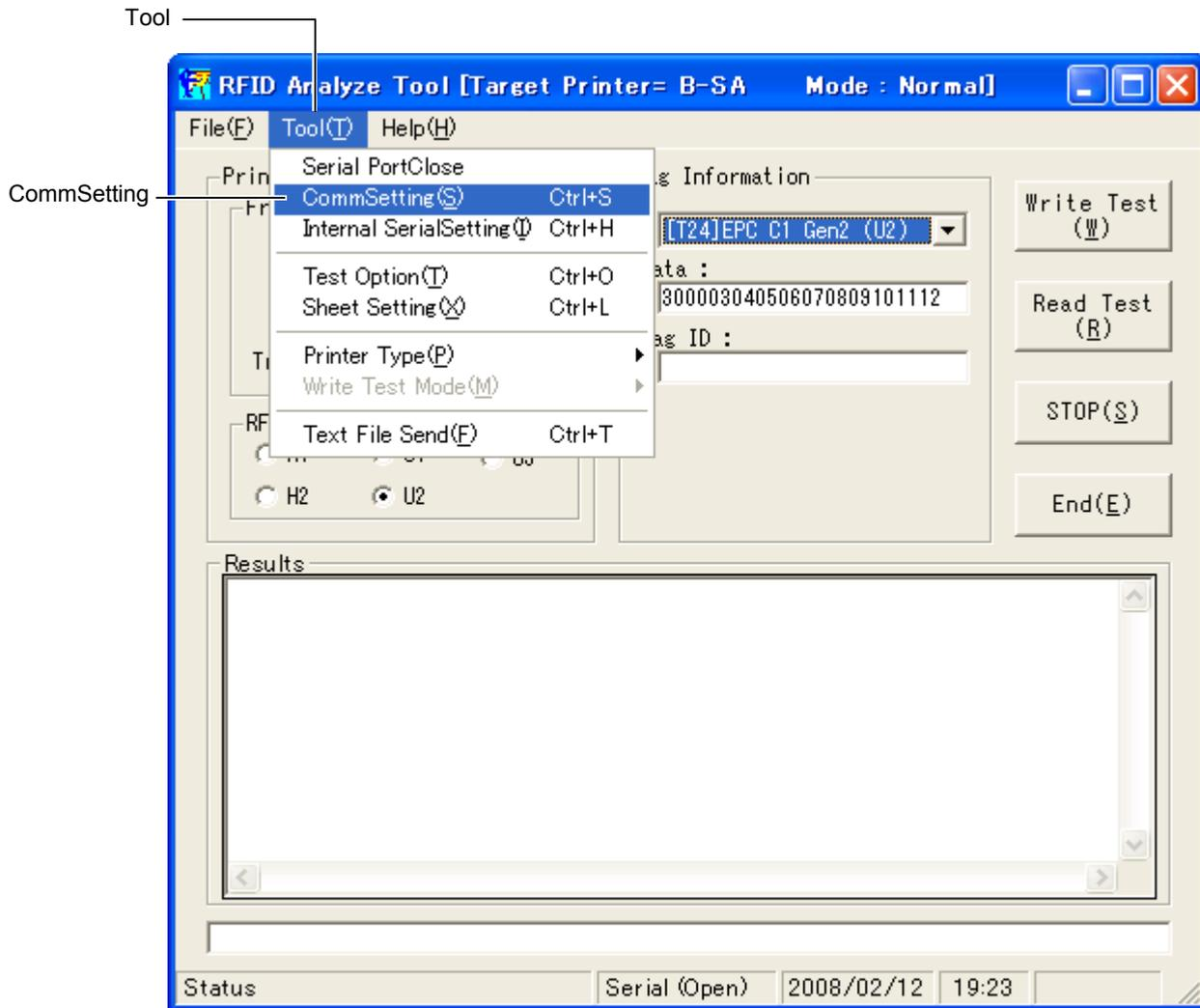
4. When the “CommSetting” screen appears, perform the serial port or LAN setting in accordance with the settings of the B-SX6T/SX8T printer.
