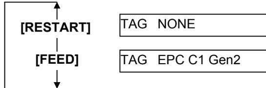
After selecting the RFID tag type to be used, press the **[PAUSE]** key.
