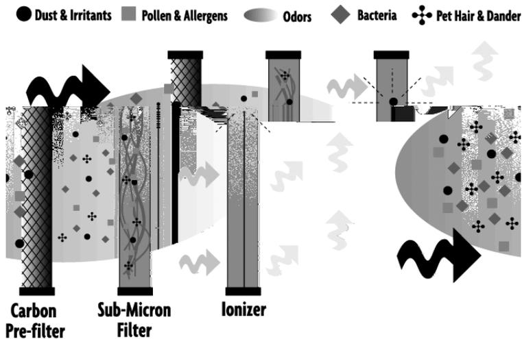
The above is an illustration of how the HEPAtch air purification system works. Dust and other irritants are pulled into the air purification system and cleaned through the HEPAtch Filter. Clean, purified air is then released into the room.
