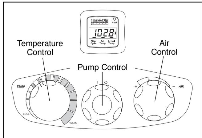
**Temperature Control:** This control is used to set the temperature of the water. The water heats at about 3.0° F per hour with the cover on. The thermostat can be set to heat the water from 70° F to 104° F. Always use an accurate thermometer to check the temperature of the water.
