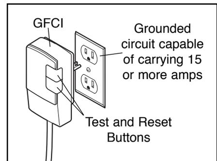
First, turn on the RENEW 207 by pressing the pump control on the console. Once the unit is running, press the GFCI “test” button. The spa should shut off. Press the “reset” button. The spa should resume normal operation. If the spa continues to run after the “test” button is pressed, the GFCI is damaged. Do not use the spa until the GFCI has been repaired or replaced by a qualified electrician.
