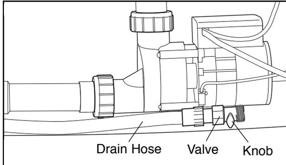
5. Open the valve by turning the knob counterclockwise. The water will begin to drain.
