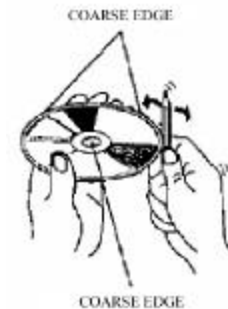
Figure 53. Rough Edges Removal
