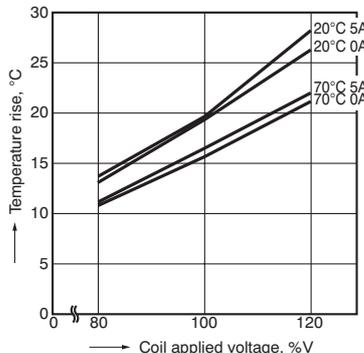
3. Ambient temperature characteristics and coil applied voltage
