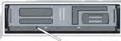
Figure 1.3 Bracket & Position of Reset Switch
