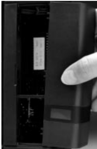
Figure 11: Access Cover removal.
