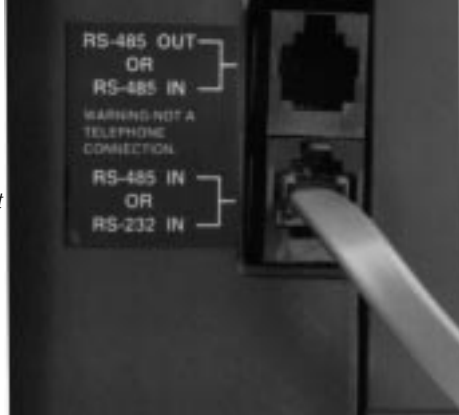
Figure 15: Data Receiver cable installation.
