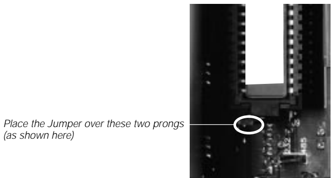
Figure 18: Installing the Two-Prong jumper.
