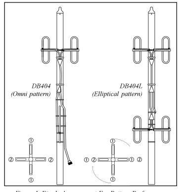
Figure 1. Dipole Arrangement For Pattern Performance
