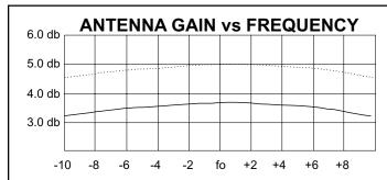
These curves illustrate the gain of the DB404 and DB404L across a 20 MHz bandwidth. Maximum gain of 3.8 dBd (DB404) and 5.0 dBd (DB404L) occur at the mid-band frequency of each range. The gain of the DB404L is shown at the pattern maximum in the horizontal plane.
