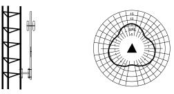
DB404 (Omni) mounted on side of tower
