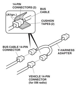
Bundle up the vehicle harness and secure it, the bus cable, and Y-harness adapter with two wire ties as shown.
