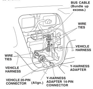
Align the Y-harness adapter 14-pin connector with the vehicle 20-pin connector and bundle up the excess bus cable. Secure it to the vehicle harness with the two wire ties.
