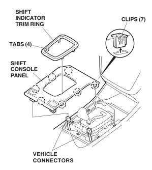
Gently remove the shift console panel (pull up to release seven clips, and unplug the connectors). 6. Move the shift lever to the N position, then remove the coin box.
