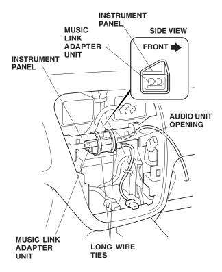
23. Secure the Music Link harness to the vehicle pipe with the two wire ties. (Align the mark you made in step 14 with the wire tie as shown).
