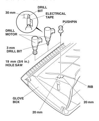
18. Route the Music Link harness DIN connector into the 19 mm hole in the direction shown, and install the grommet to the 19 mm hole.
