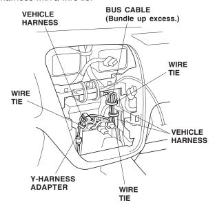
Bundle up the excess bus cable, and secure it to the vehicle harness with the two wire ties.
