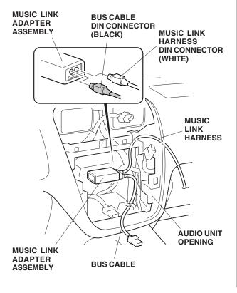
22. Secure the Music Link adapter unit onto the instrument panel with two long wire ties.
