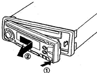
Do NOT touch the connector on the reverse side of the front panel, as doing so may contaminate the connector and cause a poor connection resulting in a malfunction.
