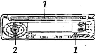
**1 Insert a disc with the labeled side upward to start CD play.**
