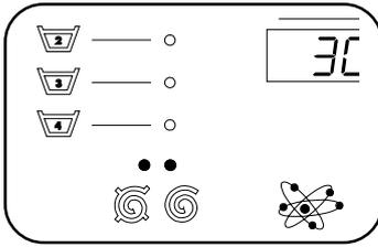
During final spin, both the **left spin-LED** (intermediate spin) will light up together with the **right spin-LED** (final spin).
