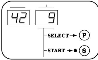
Start the wash-cycle by pressing the Start button (S) and releasing it immediately. The door is sealed and the cycle-LED lights up.
