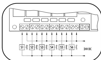
With an external tension 24V DC
