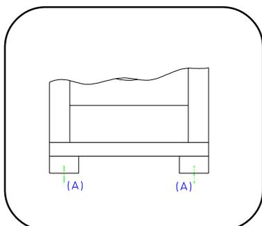
The machine must be placed on a flat, solid surface (metal base, concrete or solid ground). It is **recommended that the machine be anchored** on the provided places (A) in the base, especially in case of a plinth (see Dimensions 2).
