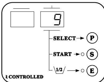
On machines with a start button, the programmer can contain up to 100 programs (0-99). The program number is displayed on the **right display**.
