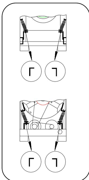
To prevent damage during transportation, the machine has been equipped with **four red transport brackets (D)** to eliminate every possible movement of the tub. After the machine has been placed level, take off the service- and the back panel to remove these transport brackets.
