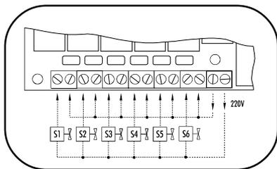
On machines equipped with a liquid soap connection, connect the wires **directly on the print board** next to the ground wire connection (option). Connect as indicated on the wiring diagram.
