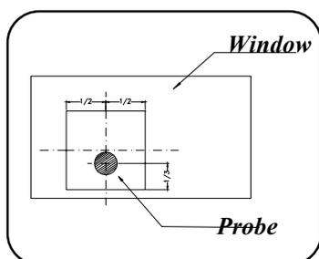
The tilt switch is mounted on the solid part of the machine. There is a window around the probe of the tilt switch that is mounted on the movable part of the machine.
