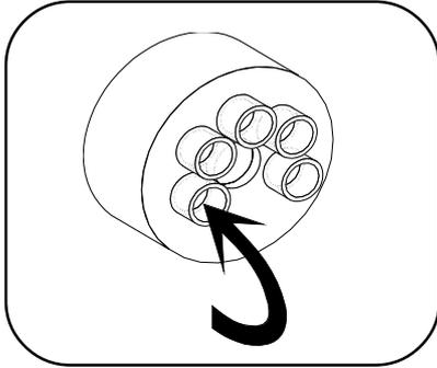
A rubber connection has been placed over the air break opening at the back of the machine. There are **5 holes** in this rubber connection, through each of which a liquid soap hose can be driven (**S1...S5**). Press the hoses until they appear well **inside the soap dispenser**.
