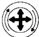
Rotate the filter while pulling straight out.
