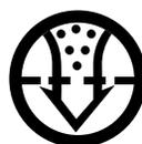
**AIR CLEANER:** With normal operating conditions, the maintenance schedule for cleaning and re-oiling the foam pre-filter is every 50 hours and replacement of the air cleaner filter element every 100 hours. More frequent servicing is required with dusty operating conditions. Refer to the maintenance section of the Engine Owner's Manual for more information.
