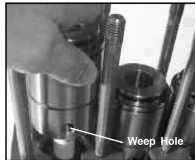
12) Check plunger surface (29B). If plunger pipe is worn out, loosen tension screws (29C) with a 15mm socket and pull off plunger pipe to the front. Clean front surface of plunger (29B) thoroughly. Apply a small drop of locktite to tension screw. Put a **new** crush washer (29D) onto tension screw. Put a thin coat of glue (Loctite) on the ring (or ceramic plunger side) and tighten screw to 265 in.-lbs.
