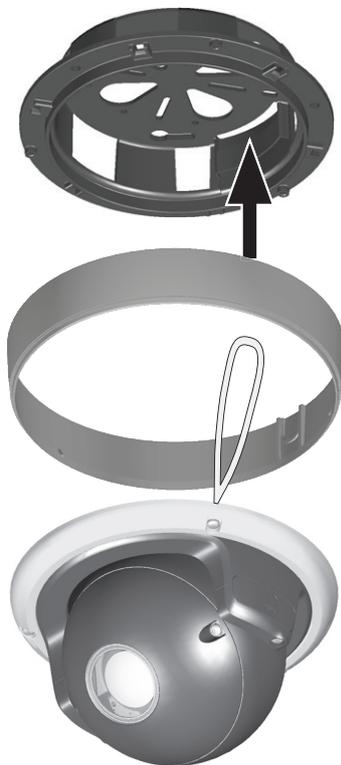
5. Place the surface mount ring over the cable tree.
