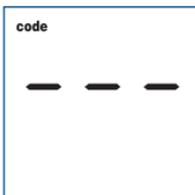
This message appears immediately after the system check if your meter has not been coded.
