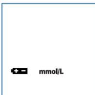
The battery sign appears on the display with the unit of measurement. The power of the batteries is getting low. You can complete about 50 more tests from the time this symbol first appears.
