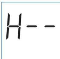
Either the ambient temperature or the meter's temperature was too high to perform a test.
