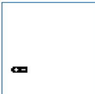
The battery sign appears on the display by itself. The power of the batteries is too low to run a test.
