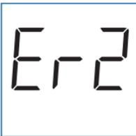
Error message could be caused by a used test strip or indicates a temporary or permanent electronics problem.
