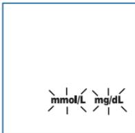
This is the first time you are using the meter. The unit of measurement is not yet selected.
