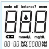
System check. Appears upon insertion of a test strip or whenever the meter is turned on. Verifies that all segments are present on the display.
