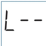
Either the ambient temperature or the meter's temperature was too low to perform a test.
