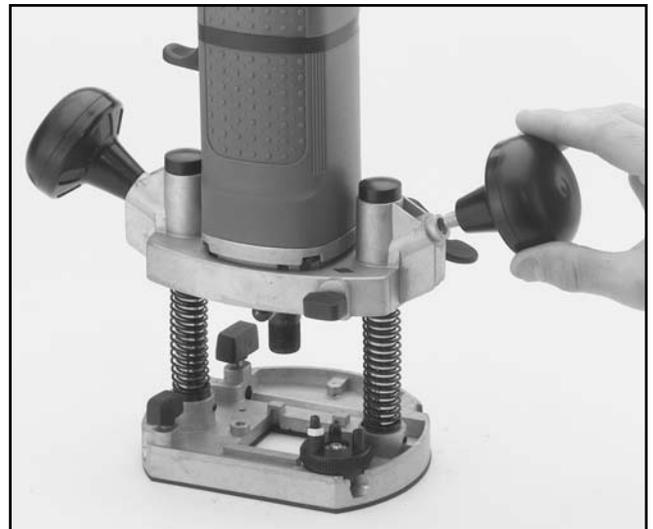
Figure 2. Installing handles.
