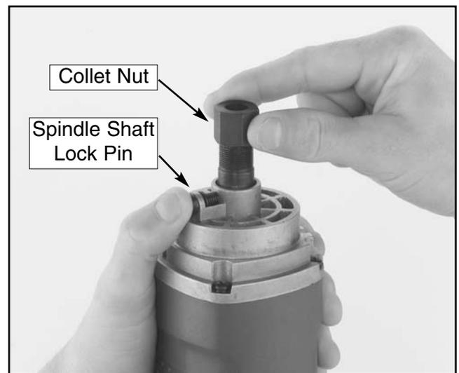
**Figure 4.** Threading collet nut onto spindle.
