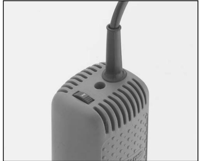
Figure 8. Spindle R.P.M. dial.
