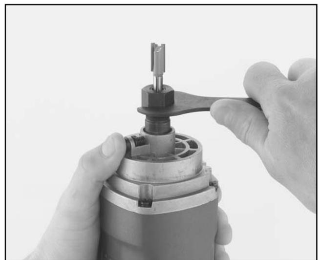
**Figure 5.** Tightening bit into router.
