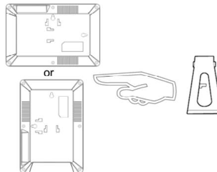
Install the stand into the hole. Photo frame can be placed horizontally or vertically.
