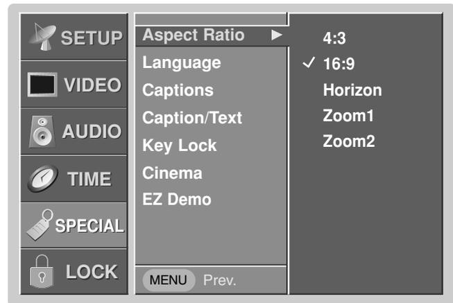
Lets you choose the way that an analog picture with a 4:3 aspect ratio is displayed on your TV 16:9 aspect ratio TV screen. When you receive an analog picture with a 4:3 aspect ratio on your 16:9 TV, you need to specify how the picture is to be displayed according to your preference.
