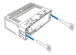
Install the sleeve into the dashboard and bend the tabs outward to fix the sleeve.
