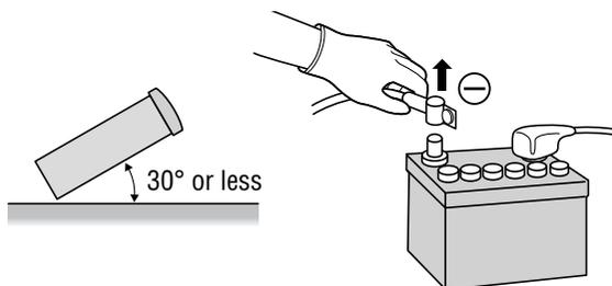
**Caution:** Do not disconnect the battery terminals of a car with trip or navigational computer since all user settings stored in memory will be lost. Instead take extra care with installing the unit to prevent shorts.
