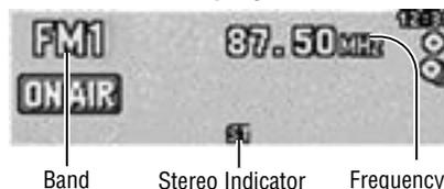
**Note:** The stereo indicator lights during reception of an FM stereo broadcast.
