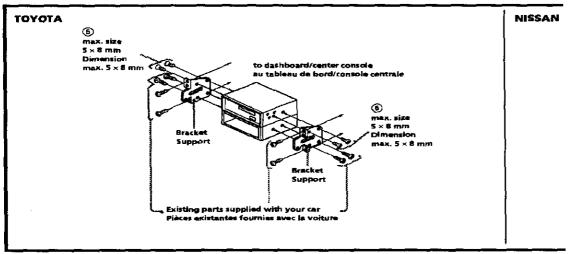
**Note**To prevent malfunction, install only with the supplied screws (§).
