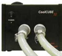
Liquid-cooled PI-MAX4 cameras can cool to a lower temperature (typically  $-35^{\circ}\text{C}$ ) than air cooling. Instead of using a fan to remove heat, these cameras incorporate a closed loop system of circulating fluid. The CoolCUBE<sub>II</sub> circulator unit continuously pumps the 50:50 mixture of room temperature ( $23^{\circ}\text{C}$ ) water and ethylene glycol. To prevent voiding the warranty, use only the circulator and hoses shipped with your system.
