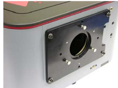
3. Mount camera to mounting plate. Rotate camera until text on back is parallel to top of IsoPlane.
