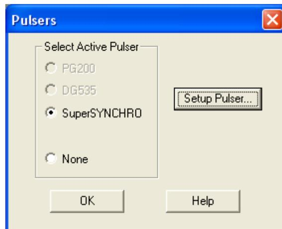
2. Select the **SuperSYNCHRO** radio button, and then click on the **Setup Pulsar...** button. The **SuperSYNCHRO** dialog is displayed, as shown in [Figure 4-7](#).
