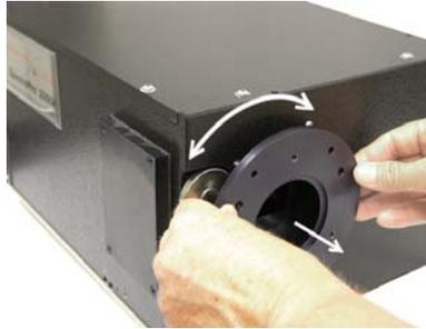
6. Finger tighten hex head screws. Leave about 1/4" thread exposed.
