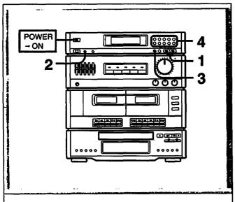
Press the DUAL MODE TUNING + or - button to tune in the desired station.
