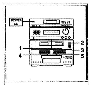
1 Insert a recorded tape into deck A and a blank tape into deck B.
