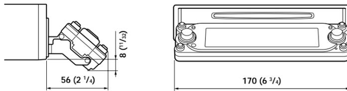
Dimensions include unit size and front panel, etc.
