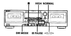
Insert the recorded cassette into deck A and a blank cassette into deck B.
