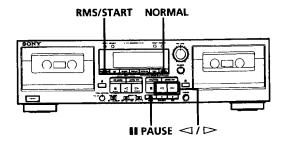
1 Insert the recorded cassette into deck A and a blank cassette into deck B.
