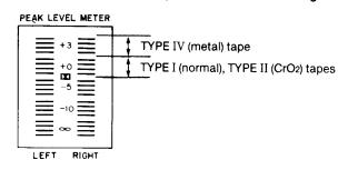
If the recording level setting is too high, the recording will be distorted, and if it is too low, the tape will produce a hissing sound.
