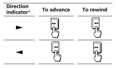
To resume playback, press the other fastwinding button partially until the locked button is released.
