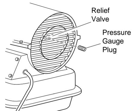
Figure 7 - Pressure Gauge Plug Removal
