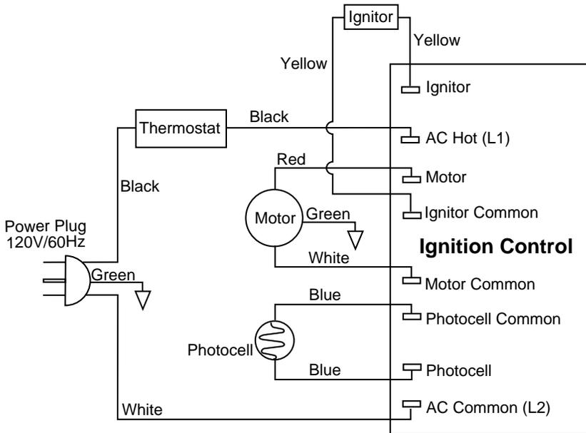
Figure 20 - Wiring Diagram
