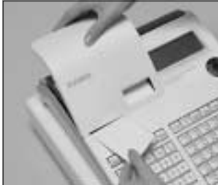
Complete Replace the printer cover, passing the leading end of the paper through the cutter slot. Tear off the excess paper.
