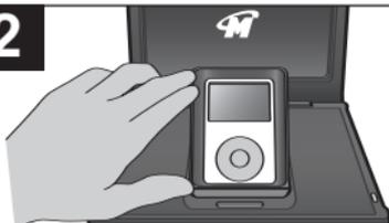
Insert the iPod into the holder. Gently push down so the connector on the iPod slides onto the connector on the Mi8000. Press the edge area of the holder down gently (as shown) until it clicks into place.
