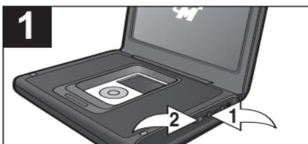
With the Mi8000 on, press the MENU button ❶; the menu will appear. To adjust the Brightness, Contrast, Sharpness, Color or Hue, select the desired option by repeatedly pressing the MENU button ❶. Then adjust the option by pressing the - / + (Volume/Setting) button ❷, followed by the MENU button ❶ again.
