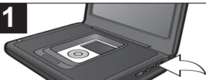
With an iPod connected (see previous page), turn the Mi8000 on by pressing and holding the Power button (if it is not on already); the Power On indicator will light green.
