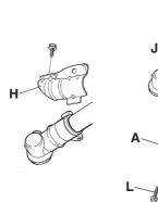
Remove the mounting plate (H). Fit the adapter (I) and bracket (J) with the two screws (K) as shown. Fit the blade guard (A) to the adapter using the 4 screws (L) as shown.
