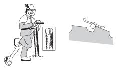
The filing angle is 15°. File alternate teeth to the right and those in between to the left. If the blade has been heavily pitted by stones it may be necessary to dress the top edges of the teeth with a flat file, in exceptional cases. If so, this should be done before filing with a round file. The top edges must be filed down by the same amount for all the teeth.
