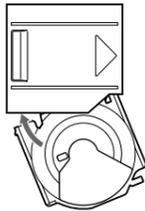
With the cut-away portion of the tray facing you, insert the right corner of the tray in the slot, then push in the left corner until it clicks.
