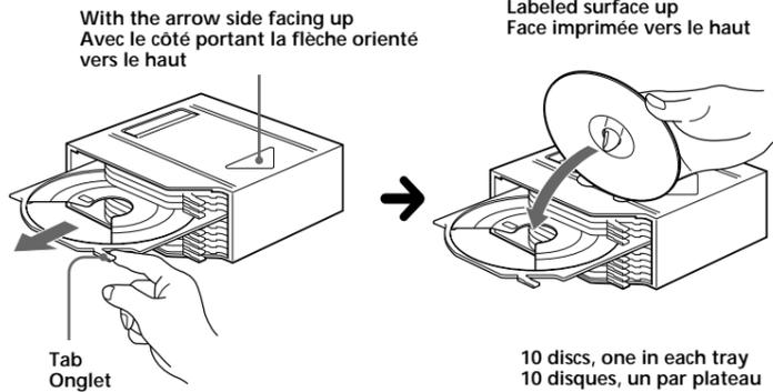
Use the supplied disc magazine or the disc magazine XA-250. The disc magazine XA-10B cannot be used with this unit. If you use any other disc magazine, it may cause a malfunction.
