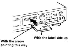
If the MD has a recorded material on it, the deck will automatically start recording from the end of the last recorded track.
