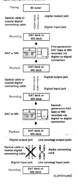
3 You can record a DAT tape or MD recorded via the DAT or MD deck's analog input jack onto another DAT tape or MD via the DAT or MD deck's digital output jack. You cannot, however, make a second-generation DAT tape or MD copy via the DAT or MD deck's digital output jack.
