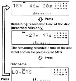
When you insert an MD, the disc name, total number of tracks, and total disc playing time appear in the display as follows:
