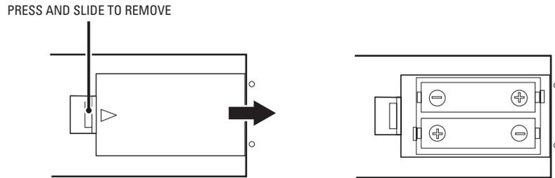
**Figure 5.** Battery Installation
