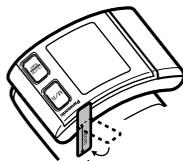
If the 2cm gauge is attached, straighten it out.
