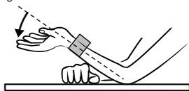
If measurements are taken with the wrist or hand in the following positions, accurate measurements may not be possible.
