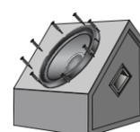
Place the subwoofer into the opening of the enclosure. Then align the screw holes of the subwoofer with the pilot holes that you drilled. Tighten the screws.
