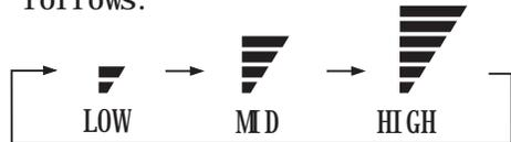
Press remote controller FAN button. For each press, fan speed changes as follows:
