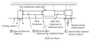
Calculate the draft and external static pressure and select the length, shape and blowout.
