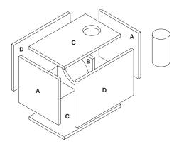
11 × 11 × 20<sup>1</sup>/4 Inches (HWD) 1.02 Cubic Feet (.50 Sealed/.52 Vented) Inside Distance from Baffle to End Panel of Sealed Side of Enclosure — 9<sup>1</sup>/2"
