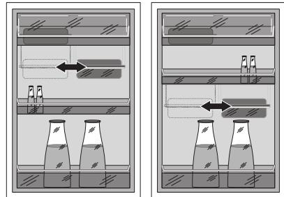
The variable box can be hung from a storage shelf in the refrigerator compartment:
