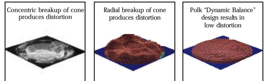
***Laser Interferometry tests produced holographic "photos" of drivers in motion. The "bad" drivers are experiencing modal breakup that results in performance-robbing resonances. A "perfect" driver would look like a cake (flat on top), more, like the photo on the right.***
