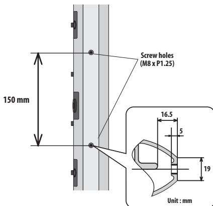
**2 Use two screws with washers to attach the stand or other fitting to the speaker.**
