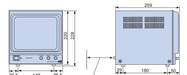
Note: Allow 80 mm behind the monitor for wiring and heat radiation. Monitor input/output uses a BNC terminal.
