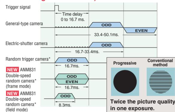
\*The shutter speed on the random camera, before exposure, needs to be set to 1/120 to 1/20000 seconds.
