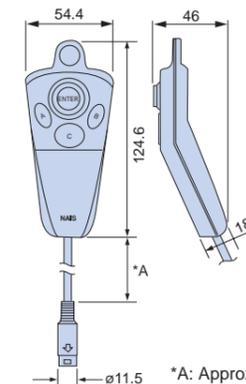
\*A: Approximated length of cable for keypad used. The cable is slightly shorter on keypads with CE marking.
