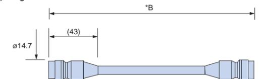
\*B: Approximated length of cable used. The cable is slightly shorter on keypads with CE marking.
