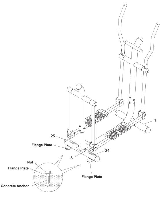
NOTE: Four concrete anchors (mounting hardware not included) are needed to secure the FRONT STABILIZER(7) and REAR STABILIZER(8) of the STAMINA® Outdoor Strider, two on each.
