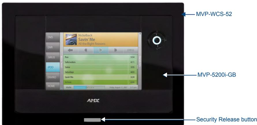
**FIG. 8** MVP-WCS-52-GB Wall Charging Station - Front
