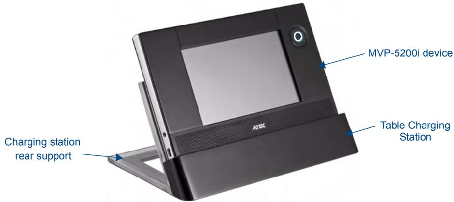
**FIG. 6** MVP-5200i in MVP-TCS-52-GB Table Charging Station
