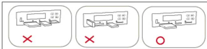
**Note:** When the system is in process, do not pull out the card.
