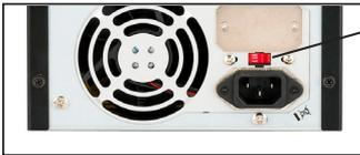
**Warning:** This product has a manually switchable power supply. **Make sure that the power supply is set to the proper voltage for your region.**
