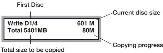
When a disc is finished copying, it will be ejected. If the Disc Spanning process is not complete, the DVD/CD Flash Copy Tower will prompt you for a new blank disc to continue the copying.
