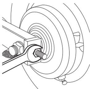
**4** Turn both adjusters the exact same amount, 1/8 to 1/4 turn at a time, to maintain the wheel alignment. Once the tension is correct, tighten the axle and brake anchor bolt.
