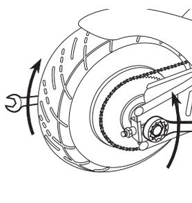
**3** Loosen the rear axle by attaching wrenches to both axle nuts and loosening counter-clockwise.
