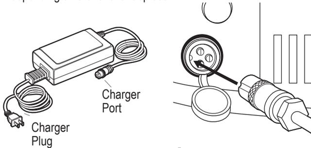
**1** Plug the charger port into the port on the chopper. The charger works with the power switch in either the on or off position.
