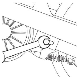
**2** Loosen the brake anchor screw (attached with the small bolt in the long slot on the left side of the frame).
