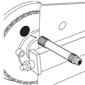
**3** Remove valve adapter immediately after inflating.
