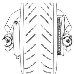
**4** Loosen the chain adjusters about 3-4 turns. Be sure to loosen both adjusters an equal number of turns.
