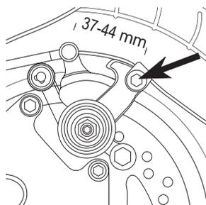
**2** If the brake has too much slack, loosen the rear anchor bolt and pull the brake wire tighter. The distance of the brake wire between the end of the cable and the anchor bolt should be between 37-44 mm.
