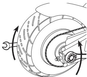
**1** Loosen the rear axle by attaching wrenches to both axle nuts and loosening counter-clockwise.
