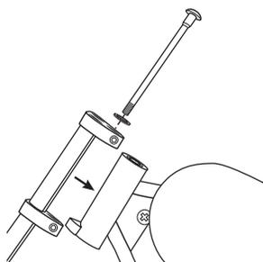
**2** Slide the fork into position and insert the steering bolt. The bolt must go through the washer and spacer sleeve and between the steering bearings inside the frame.
