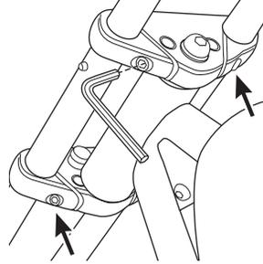
**3** Tighten all four pinch clamp screws (two in the upper and two in the lower crown).
