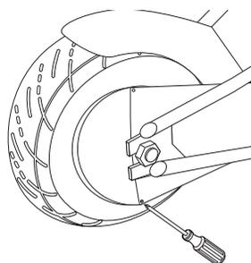
**1** Loosen screw and remove chain guard.
