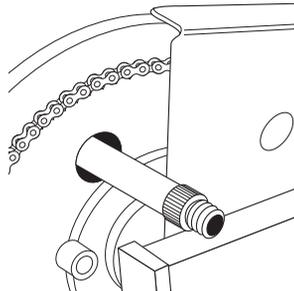
**2** Align the access hole in the drive sprocket with the tire valve. Thread the adapter completely onto the valve and attach the pump. Inflate to the PSI indicated on the tire sidewall.
