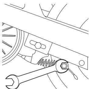
**1** Loosen and disconnect the brake cable anchor.
