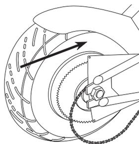
**3** Slide the wheel forward to slacken the chain and disengage the chain from the wheel sprocket and motor sprocket.
