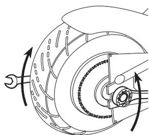
**2** Loosen the rear axle by attaching wrenches to both axle nuts and loosening counter-clockwise.
