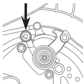
**3** If the brake rotor is dragging on the brake pads use your fingers to twist the calliper adjuster in either direction until rotor is centered between pads.
