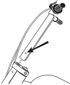
**1** Press the spring buttons on each side of the handlebars and tap the bars until the spring buttons slide inside and engage the corresponding holes in the fork.
