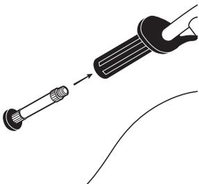
**4** Place the adapter back into the handlebar grip for later use.
