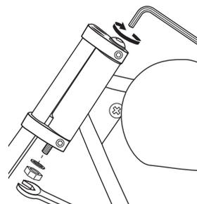
**3** Install washer and nut onto steering bolt. Tighten until snug, then back off slightly to allow the steering to rotate freely with no binding or end-play.
