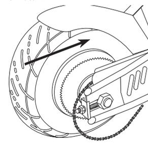
**5** Slide the wheel forward to slacken and disengage the chain from the wheel sprocket and motor sprocket. **(Note: Your hands will get greasy doing this.)**
