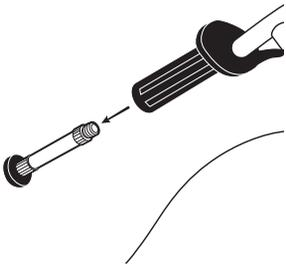
**1** Use the special valve extender/adapter supplied. This item is concealed in the grip on the speed control side of the handlebar.
