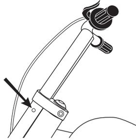
**2** When correctly engaged, the handlebars will not disengage from the fork.
