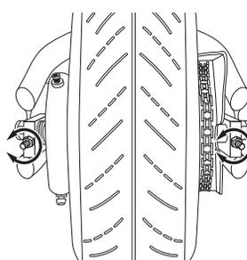
**3** Tightening the adjusters clockwise tightens the chain; loosening the adjusters counter-clockwise will relax it. When loosening the adjusters, you will have to nudge the axle forward by tapping the wheel with your hand to relax the tension on the chain.
