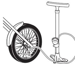
**1** Using a bicycle style tire pump equipped for a Schrader-type valve, inflate the front tire to the PSI indicated on the sidewall of the tire.
