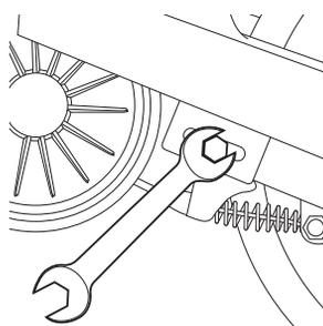
**2** Loosen and disconnect the brake housing anchor. **Note:** Pay attention to the location of the parts for when you reinstall.
